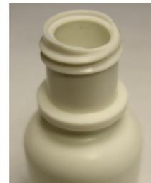
Seal Surface Defect Examples – Common Benefit of Leak Testing
