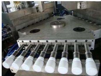
Injection Blow Molded (IBM) Bottles
