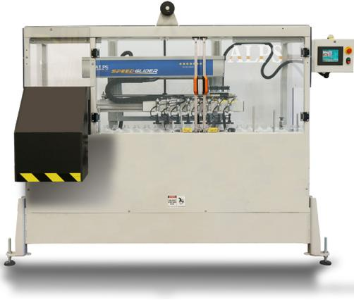
The **Speed-Glider** family of machines are applicable for higher speed, or higher sensitivity, applications where single-station machines are not fast or sensitive enough. The **Speed-Glider** uses a Timing Screw for each bottle, to space the bottles for leak testing and to provide positive bottle handling. The machine incorporates a single servo-driven slide to match the slide speed to the timing screw.
